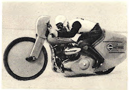
A broadside view of the streamlined motorcycle which set a new speed mark at Daytona Beach, Fla. Streamlined rear also adds to stability of the machine at high speeds.
