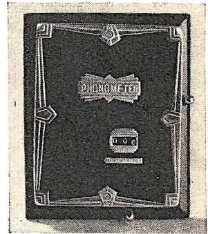
New device keeps visible record of all outgoing calls from any household or office telephone.
