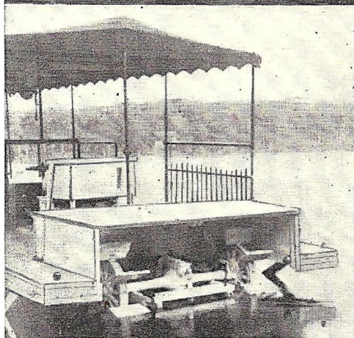
This 25-passenger sightseeing boat (top) was constructed by H. G. Meigs, of Milwaukee, Wis. Lower photo shows how paddle wheels are attached to auto rear-end to propel the craft.
