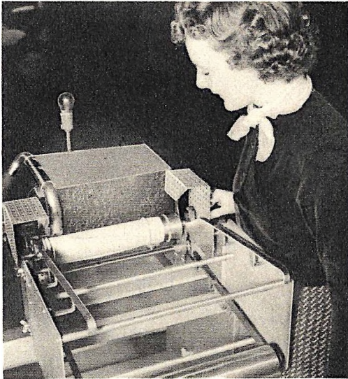
With this new device, colors may be transmitted by telegraph. Each color has its own characteristic graph curve. No two curves are exactly alike unless they are for the same color.
