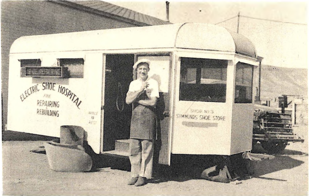
Starting with the idea of having a short vacation during which he could earn enough money to cover expenses, Ivan Symmonds mounted shoe repairing machinery in his home-built trailer. The novel shop attracted so many customers that he has been traveling for three years, doing business in towns en route. A 75-foot cable connects machinery with nearby electric lines.
