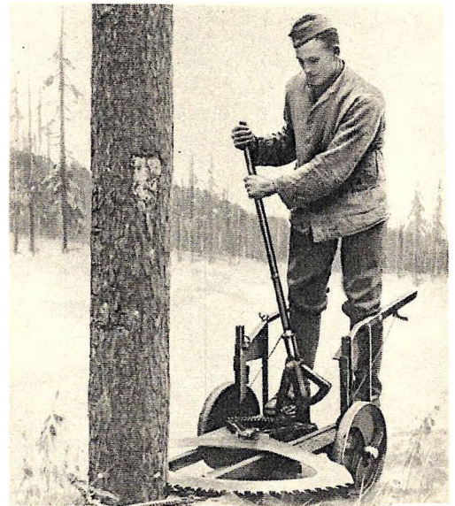
Lever-operated saw cuts close to the ground and is operated by workman in standing position. Gears transfer power from lever to semi-circular saw blade. Spring maintains blade pressure.
