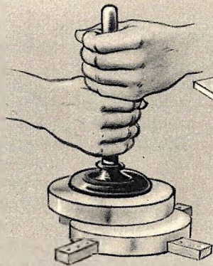
Above — Diagram showing method of grinding mirror by hand. A "plumber's friend" is used as a handle for the mirror. A glass "tool" is under the mirror. Blocks of wood are used to hold the "tool" in place during grinding operation.
