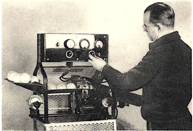
Fruit passing through electrically operated device capable of determining, by resistance test, whether fruit is frosted and dried or decayed. Damaged pieces are shunted into discard.
