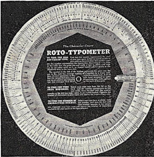
Circular slide rule for solving problems involving type, cuts and space to be filled. Device supplies easy and rapid means of obtaining answers to questions arising in the printing art.
