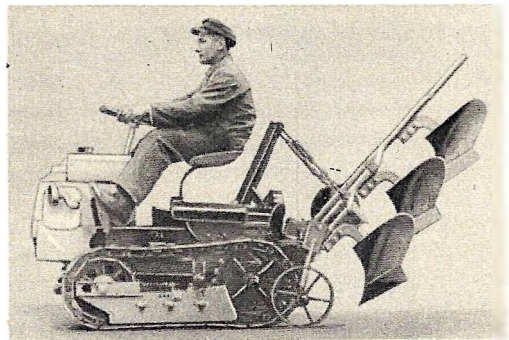
Designed especially for farm work where narrow strips of land are to be worked, this "crawler" is equipped with an 8-horsepower gasoline engine and has great tractive power.
